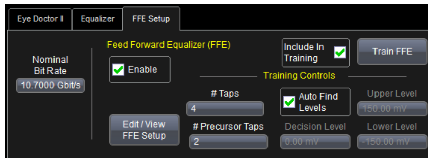
Figure 33 - Screen capture of SI Studio's FFE control window
