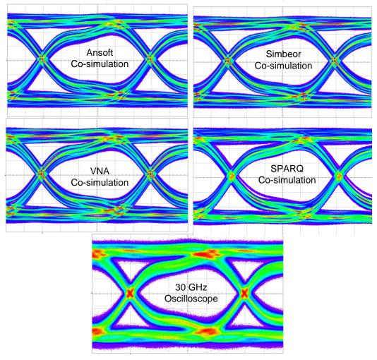
Figure B1: For visual comparison of eye diagrams predicted with Co-simulation (real input stimulus) with emulated "channel", and last a measure eye-diagram
