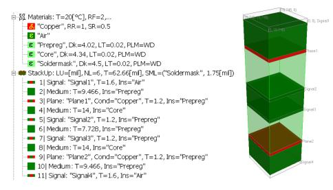
Figure 4 Fabrication vendor's CMP-08 board materials and stackup in Simbeor 2011
