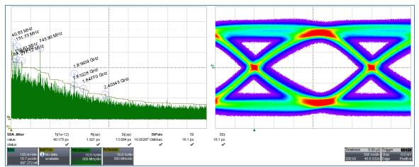
Figure 29 - Using an FFE equalizer to open the eye (same tap values), the jitter and eye diagram can still be calculated. Synchronous PRBS31 aggressor (McMorrow). This is a simulation of the "aggressor-on" case. Note the ISI and DDj do not increase ... which is expected since they are systematic. Note also that the Rj value increases by about a factor of 2.
