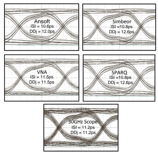
3 inch Differential Stripline Comparison of Noiseless Eye Diagrams, ISI and DDj jitter figures.
