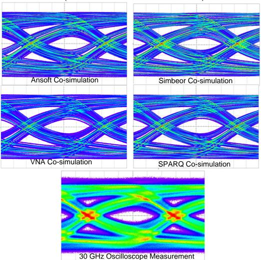
Figure B3: 4 co-simulations and one direct oscilloscope measurement for the 11-inch differential stripline.
