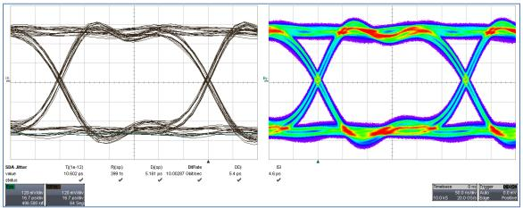
Figure 17 - Direct measurement of Centellax<sup>™</sup> (TG2P1A) Generator with no test structure with deembedded cables (both pairs used in other measurements). The ISI measurement is 4.6ps and DDj is 5.4ps ... a surprise since they are less without the cables de-embedded
