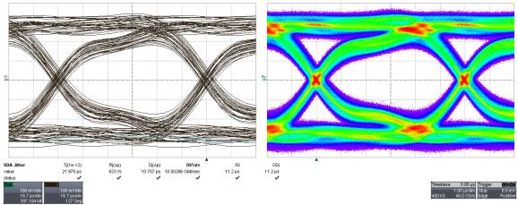
Figure 15: Direct measurement of Centellax<sup>™</sup> (TG2P1A) Generator through 3"differential stripline with cables, connectors and launches de-embedded. The ISI measurement is 11.2ps, whereas the simple prediction using an ideal stimulus was 5.8ps. How is the apparent difference explained?
