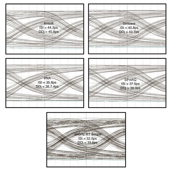
Figure 20 - 4 Co-simulations and 1 direct measurement of the "noiseless" eye-diagram for the 11" differential stripline structure, showing good agreement between the deterministic jitter for all cases based upon measurement (i.e. scope, VNA, and SPARQ/TDNA). The modeled values are consistently higher than the measured cases.
