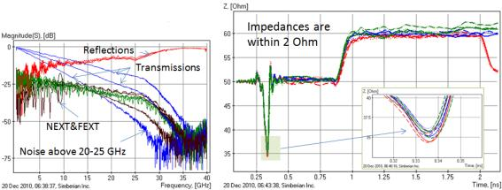
Fig. A.2. Measured single-ended S-parameters for 3 test fixtures with coupled strip line segments (left graph); TDR profile for all coupled strip line structures (right graph, computed with rational macro-model of S-parameters).
