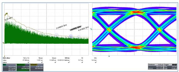
Figure 31 - Measurement of PRBS7 (by accident) Aggressor, with a PRBS7 Victim ... FFE 5 taps, 2 pre-cursor, as for simulations above. Note the Rj unexpectedly did not grow with the cross-talk case.
