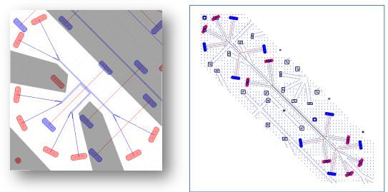
Figure 6 - Layout of Neves Pathological Test Structure (left), and McMorrow Coupler (right)
