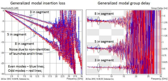
Fig. A.4. Measured GMS-parameters of strip line segments extracted from regular Sparameters of 3 in, 6 in and 8 in test fixtures.
