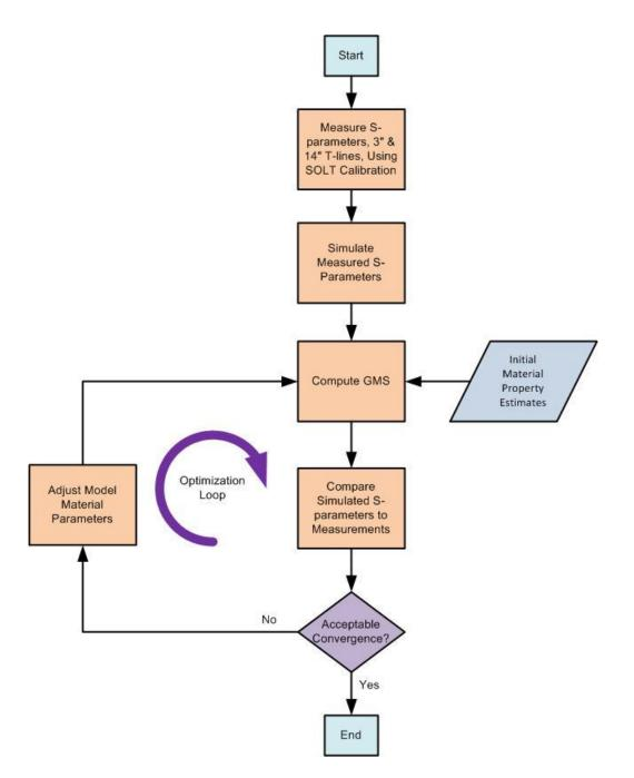
Figure 13 – New GMS method of material extraction.
