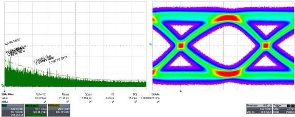
Figure 34 - Measurement of synchronous PRBS31 Aggressor, with a PRBS7 Victim ... FFE 5 taps, 2 pre-cursor, as for other cases which are equalized above. The Rj does increase, and by about a factor of 2, like it did for the simulation of equalized data.
