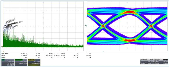
Figure 28 - Using an FFE equalizer to open the eye, the jitter and eye diagram can still be calculated for (McMorrow) simulation. This is the control or "no aggressor" case, and it is a simulation.
