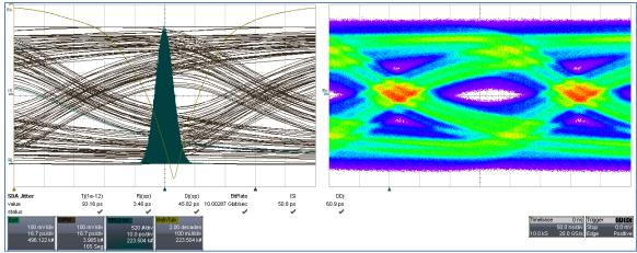
Figure 27 - Direct measurement of the victim differential pair for the "McMorrow Coupler". The victim is PRBS7 and the aggressor is PRBS31 phase locked to the same clock, but at arbitrary phase. (Cables are de-embedded even though they are high quality)
