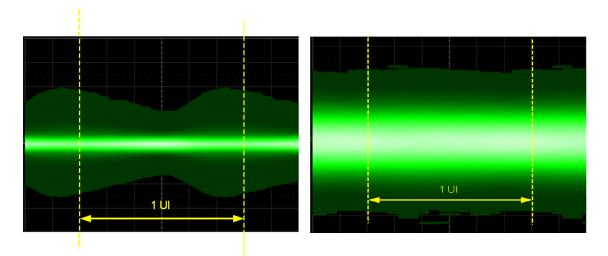
Figure 32 - Display of the phase dependent noise (left) on the victim channel for the PRBS31 Aggressor and PRBS7 victim simulation. This display is "flat" for the control cases (right), and merely inflated for the Measured cross-talk case, indicating that the Aggressor channel was not was not phase locked, as it was believed for the measurement case (while the aggressor was certainly synchronized for the simulation case). Vertical scale is note the same.
