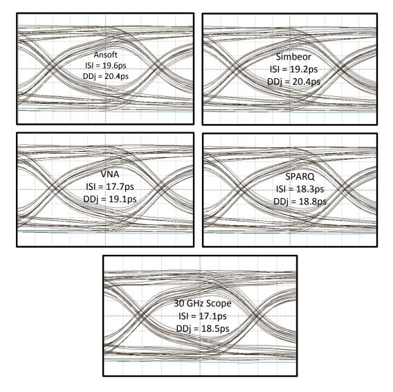
Figure 19 - 4 Co-simulations and 1 direct measurement of the "noiseless" eye-diagram for the 6" differential stripline structure, showing good agreement between the deterministic jitter for ALL of these cases with measurement and with each-other. (Note: the first printing of this paper showed a case which had poor agreement, which was corrected)
