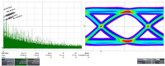
Figure 33- Measurement of No Aggressor, with a PRBS7 Victim ... FFE 5 taps, 2 pre-cursor, as for other cases which are equalized above. The Rj is 1.23ps, and is slightly larger than the 1ps Rj for the original PRBS7 generator.
