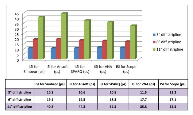
Table 4 - : ISI values for 4 Co-simulations and 1 direct measurement of the "noiseless" eye-diagram for the 3", 6" and 11" differential stripline structures, showing good agreement for all cases except for the 11" case.
