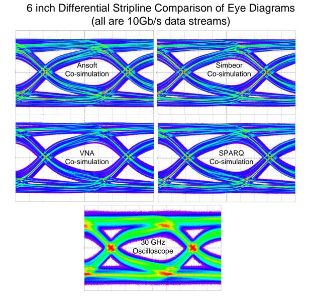
Figure B2: 4 co-simulations and one direct oscilloscope measurement for the 6-inch differential stripline.
