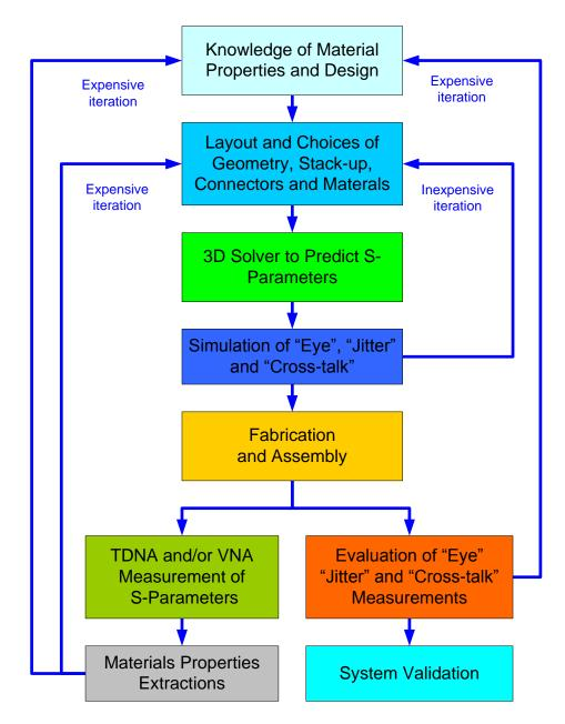
Figure 2: A simplified block description of the design process of a high-speed digital channel
