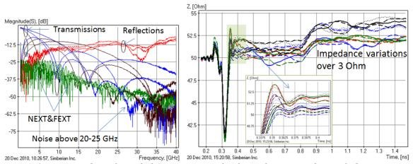
Fig. A.1. Measured single-ended S-parameters for 3 test fixtures with coupled microstrip line segments (left graph, parameters in the first row of S-matrix are shown); TDR profile for all coupled strip line structures (right graph).
