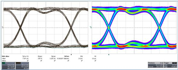
Figure 16 - Direct measurement of Centellax<sup>™</sup> (TG2P1A) Generator with no test structure both pairs of cables used in other measurements). The ISI measurement is 3.5ps all by itself, and DDj is the same.
