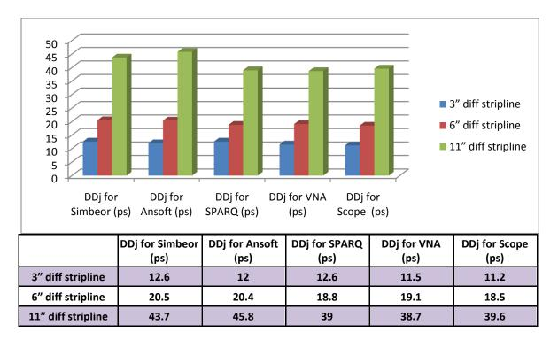
Table 5 - DDj values for 4 Co-simulations and 1 direct measurement of the "noiseless" eye-diagram for the 3", 6" and 11" differential stripline structures, showing good agreement for all cases.
