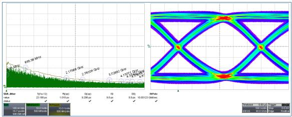
Figure 30 - Measurement of PRBS7 Victim ... FFE 5 taps, 2 pre-cursor, as for simulations above. This is not a simulation. It is the control case (no Aggressor). Approximately 1 million UI.
