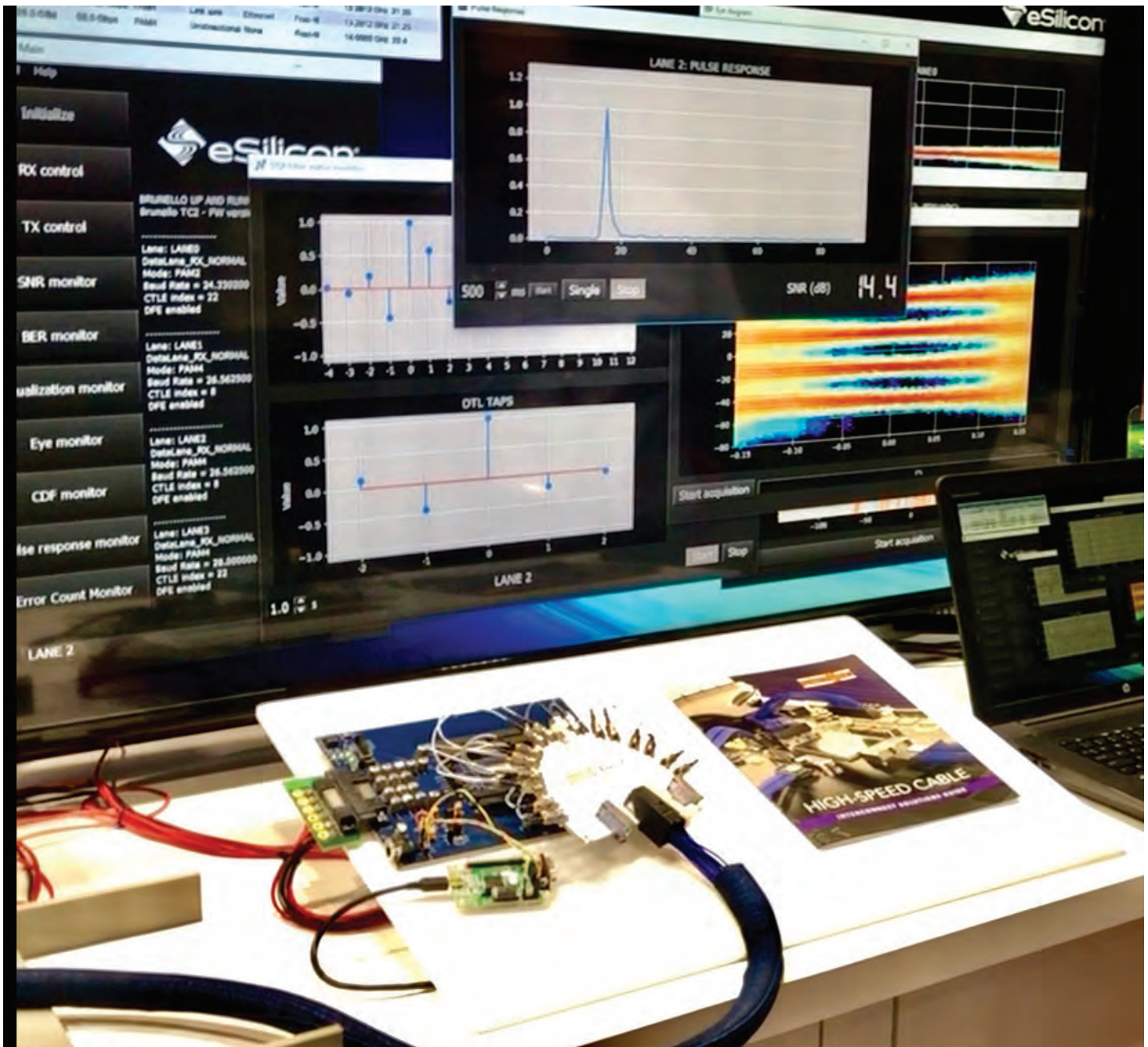
Figure 4. Real-time SerDes test data display
