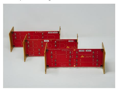
The **ISI–224** Loss Modeling kit includes the 3 assembled and tested ISI platforms shown above, s-parameters, User Guide, and ruggedized case.
