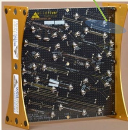
Example using Via-path trace – Via, mimics connector and breakout field
