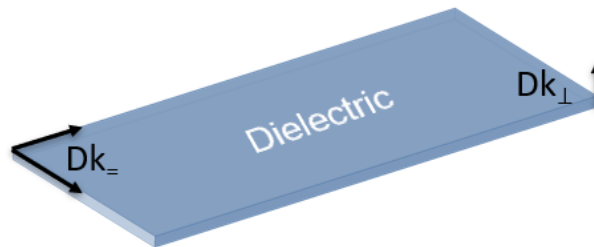
Figure 19 Dielectric material with indication of in-plane and out-of-plane Dk values
